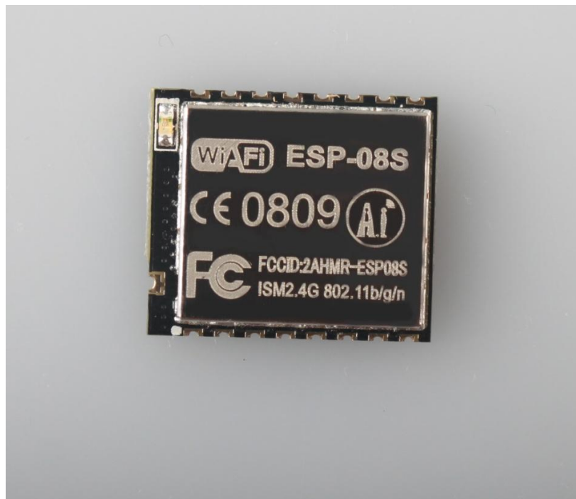
Figure 2 [Module Pin Counts, 17 pin, 16mm x 18.5mm x 0.8mm]
